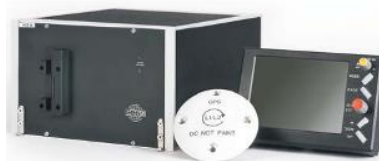
Image showing the Central Computer Unit (CCU), the Command & Display Unit (CDU) and the TSOed L1/L2 GPS antenna.
